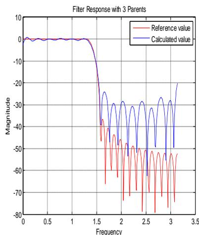
Fig ,6 Magnitude Response of FIR Filter using three Parents at 500 generations with 4 attempts
