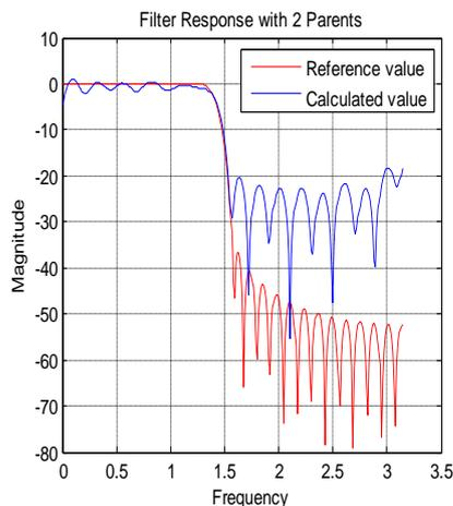
Fig 5: Magnitude Response of FIR Filter using two Parents at 500 generations with 4 attempts
