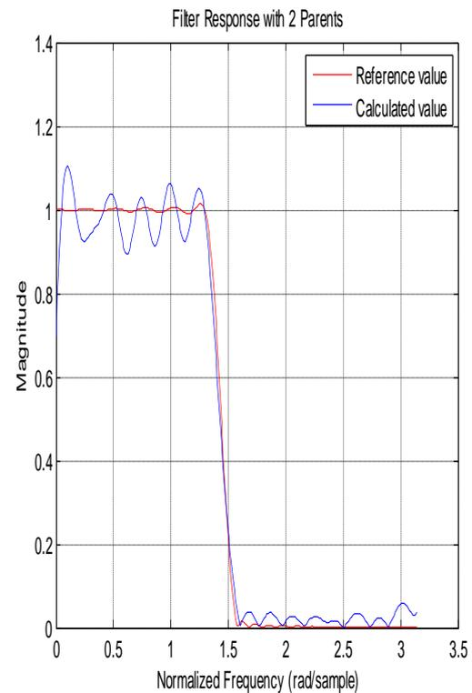
Fig 3: Magnitude Response of FIR Filter using two Parents at 600 generations with 11 attempts
