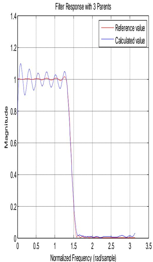
Fig 4: Magnitude Response of FIR Filter using three Parents at 600 generations with 11 attempts
