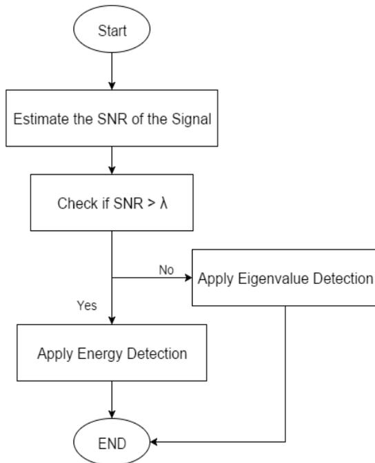
Fig. 1. Flow Diagram of Adaptive Spectrum Sensing
