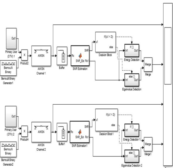
Fig. 8. Matlab Simulink schematic of adaptive spectrum sensing method
