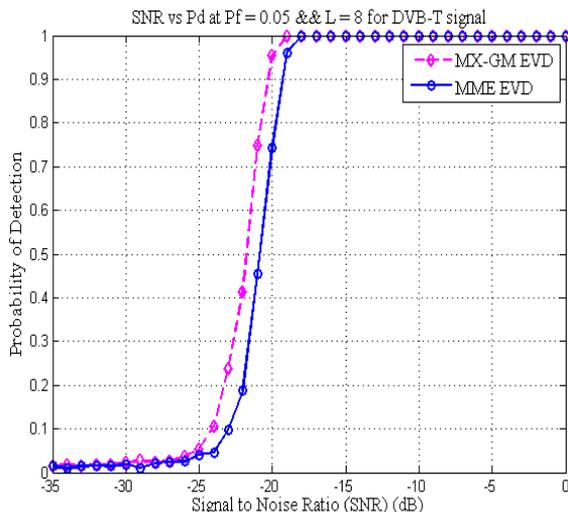
Fig. 6. Comparison of MME and MX-GM EVD method
