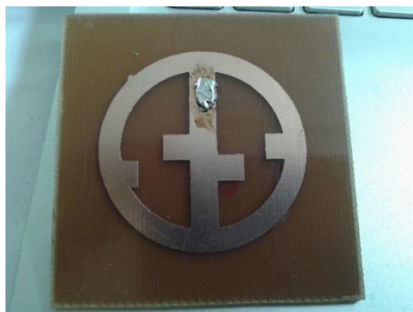
Fig. 8 : The hardware design of the proposed antenna
