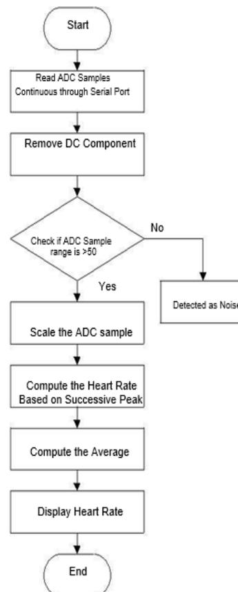
Fig. 2: Flowchart chart of sensor data processing
