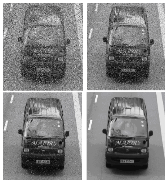
Fig.4 Low-pass filtering technique. (a) Image is corrupted with 50% of noise density (b) Using of 7 X 7 average filter (c) Using of 9 X 9 average filter (d) Original Image
