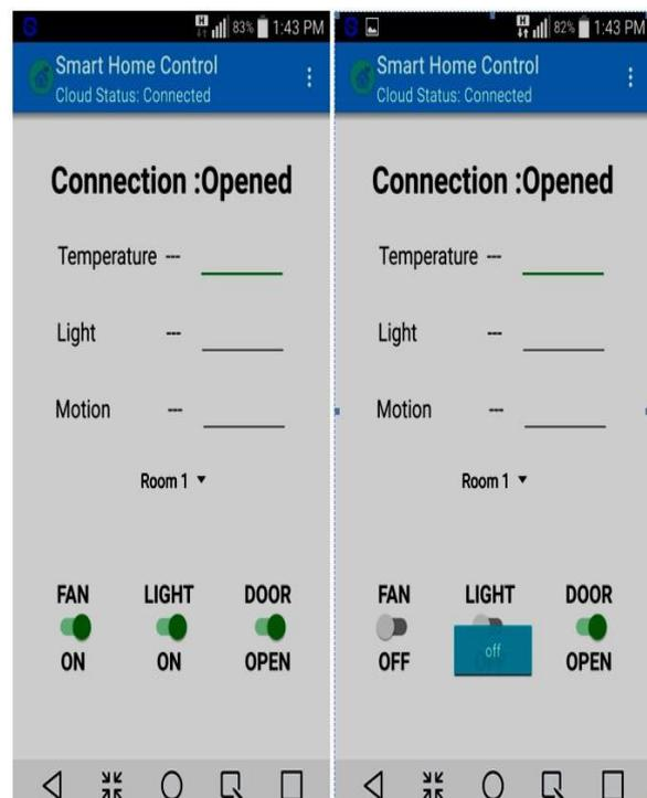
Fig. 14. Screenshots of Room 1 Control ON/OFF of the smart home application.
