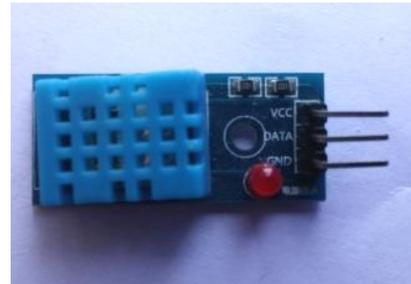
Fig. 9. Temperature and Humidity Sensor
