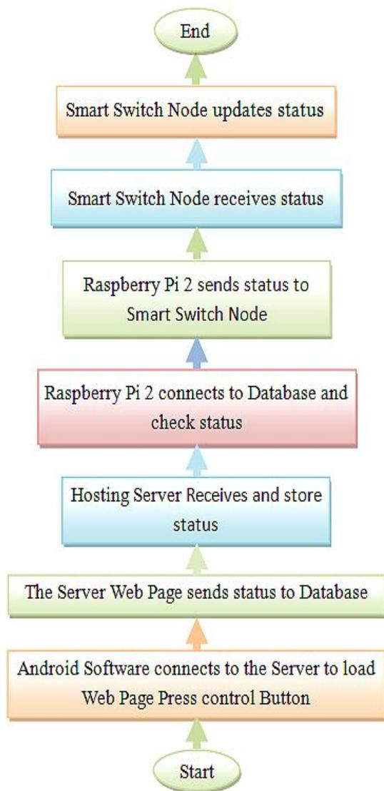
Fig. 15. Flow chart for Android app sends status to smart switch node.
