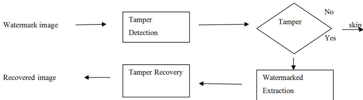
Block Diagram1: Tamper Detection
