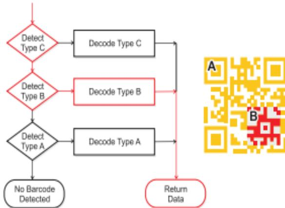
Figure 10. Attack: The inner barcode type is always detected before the outer one
