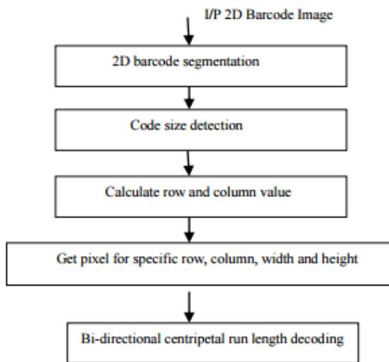
Figure 7. Decoding 2D barcode
