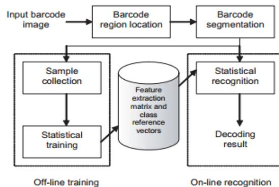
Figure 3. Diagram of the bar code decoding system
