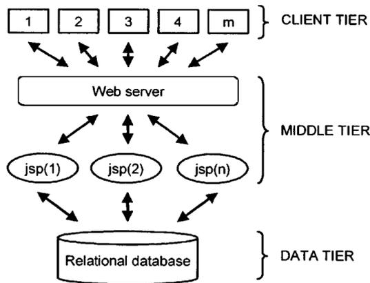
Fig 2: Multi-tier software architecture for programming
