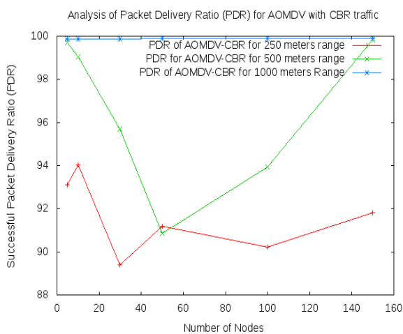
Figure 32: Overall Analysis of PDR of AOMDV over CBR.
