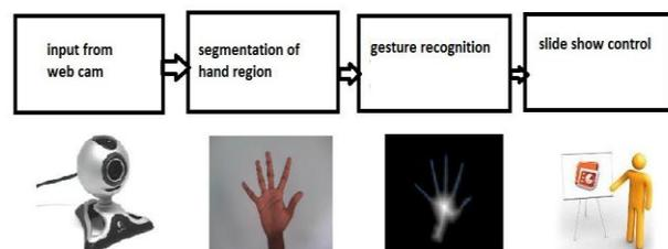
Figure1. Architecture for hand gesture recognition
