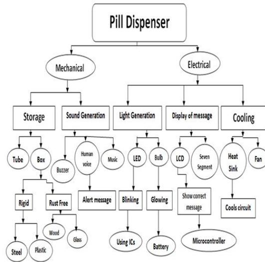
Fig. 8 Function Means tree
