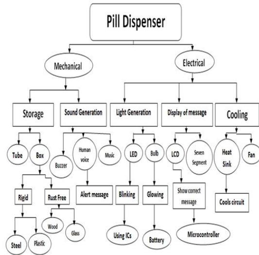
Fig. 8 Function Means tree
