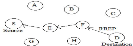
Fig. 7: Route Reply from Source to Destination in AODV
