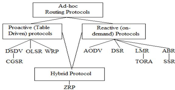
Fig. 3: Family Diagram of Proactive, Reactive and Hybrid Routing Protocol.
