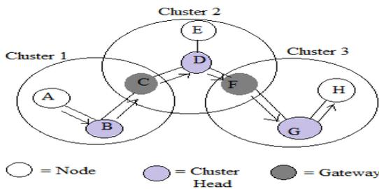
Fig. 5: Communication Diagram of CGSR via Cluster Head and Gateway.
