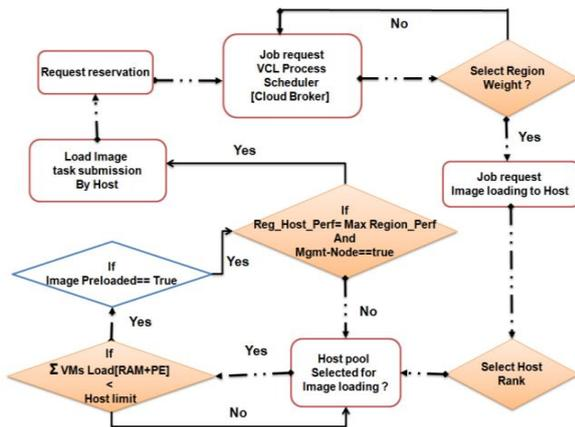
Figure 2: Flowchart of the Improved VCL scheduler algorithm
