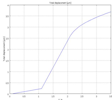
Figure 9: Displacement Vs Voltage Curve PTFE.
