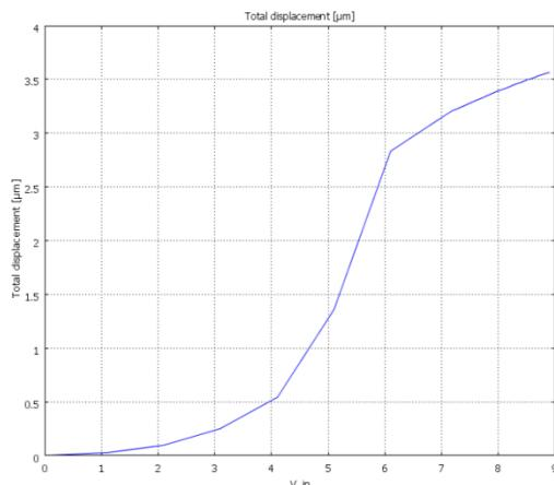
Figure 7: Displacement Vs Voltage Curve PMMA.
