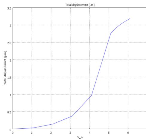
Figure 8: Displacement Vs Voltage Curve SU-8.
