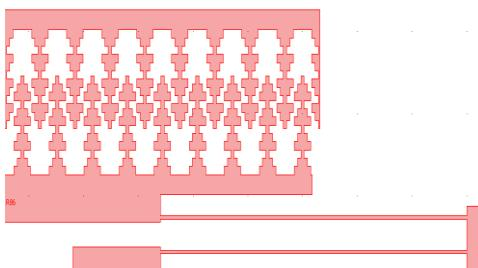
Figure 3: Staircase Micro tweezers.
