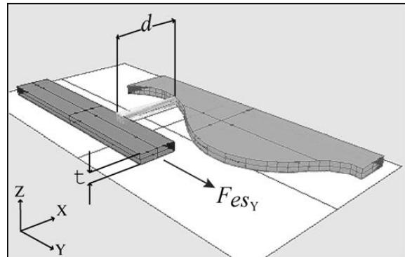
Figure 4: Variable Gap Comb Fingers [10].
