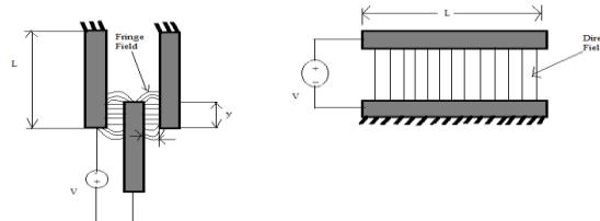
Figure 1(a): Interdigitated Comb Figure 1(b): Parallel Plate Comb
