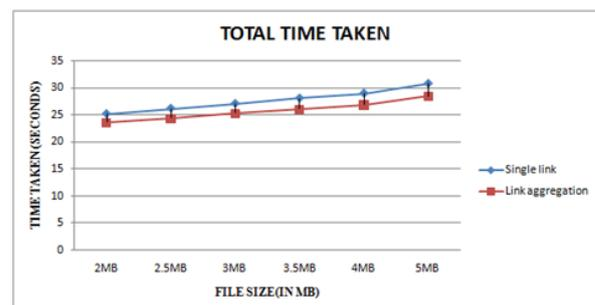
Figure 6: Total time taken for both link aggregation and single link using UDP.
