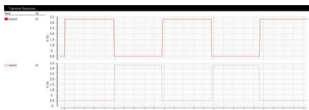
Fig. 8 Non- overlapping clock pulses
