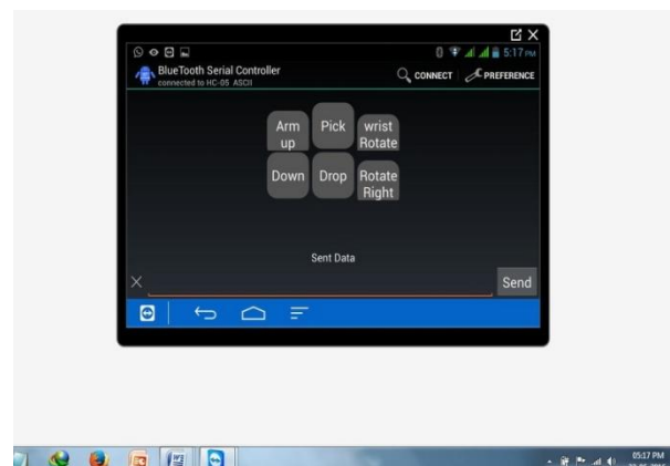
Fig. 6: Cropped image showing how the mobile screen is to control the robot arm is seen on the laptop
