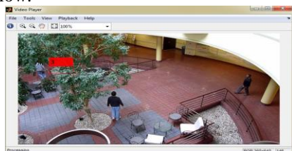
Figure 4.8: Count is estimated from the image frame containing three people in image frame.
