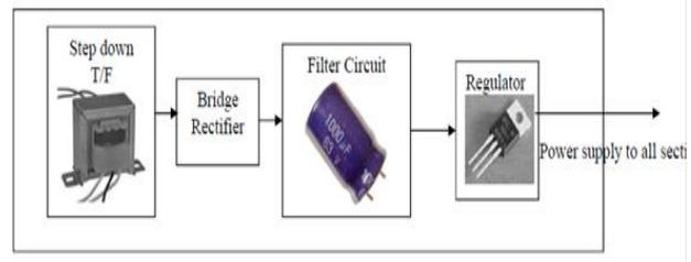
Fig: Regulated Power supply
