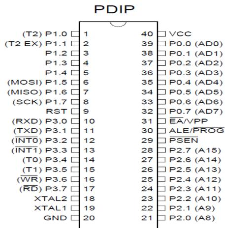
Fig: Pin diagram of microcontroller
