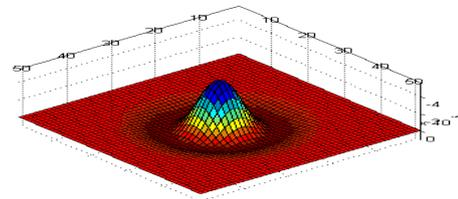
$$\nabla^2 G(x, y, \sigma) = \frac{\partial^2 G}{\partial x^2} + \frac{\partial^2 G}{\partial y^2}$$
