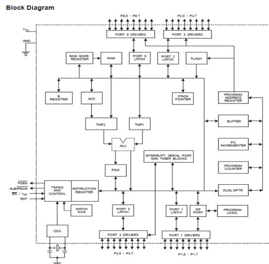
Fig: Block diagram of microcontroller
