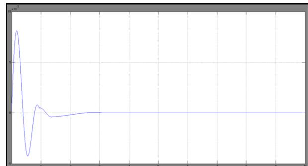
Fig-9(c) Change in diesel power generation for the step load change of 2% (0.02p.u.)
