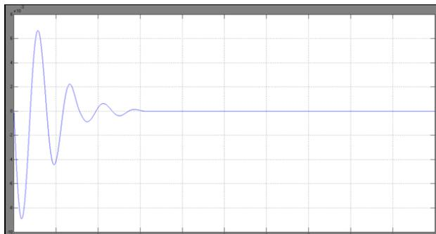
Fig-9(d) Change in hydro power generation for the step load change of 2% (0.02p.u.)
