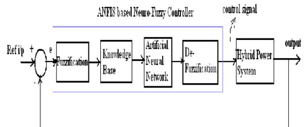
Figure-7 Block diagram of ANFIS based Neuro-Fuzzy Controller
