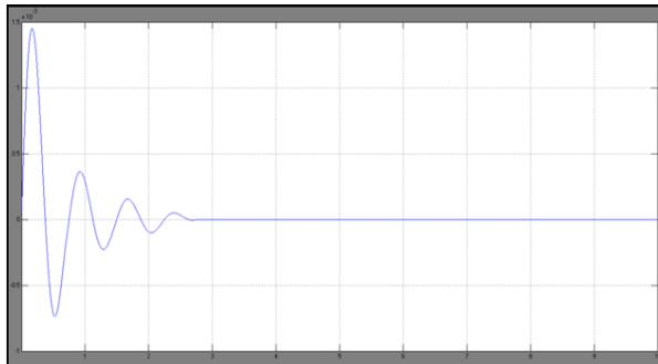
Fig-10(a) Change in frequency for the step load change of 4%(0.04p.u.)
