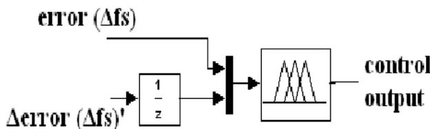
Figure-4: Block diagram of Fuzzy logic controller.
