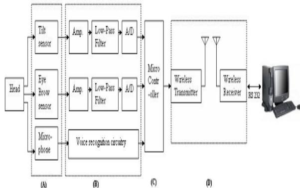
Fig.1. the block diagram representation of the tilt sensors-controlled computer mouse interface
