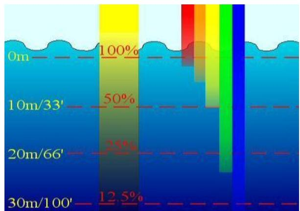
**Fig 5** Light Absorbed by water
