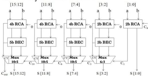
Fig.3 16-Bit Modified Carry Select Adder Schematic
