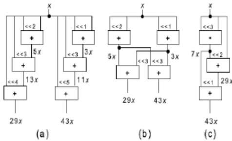
Fig.2 29x and 43x Shift-adds implementations (a) without partial product sharing and with partial product sharing. (b) Exact CSE algorithm. (c) Exact GB algorithm
