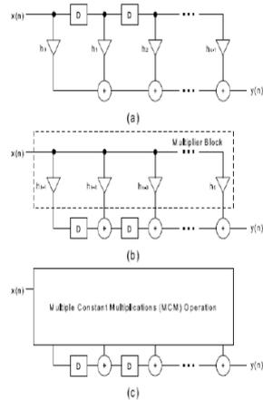
Fig.1 FIR filters (a) Implementation in Direct form. (b) Implementation in Transposed form with generic multipliers. (c) Implementation in Transposed form with an MCM block.
