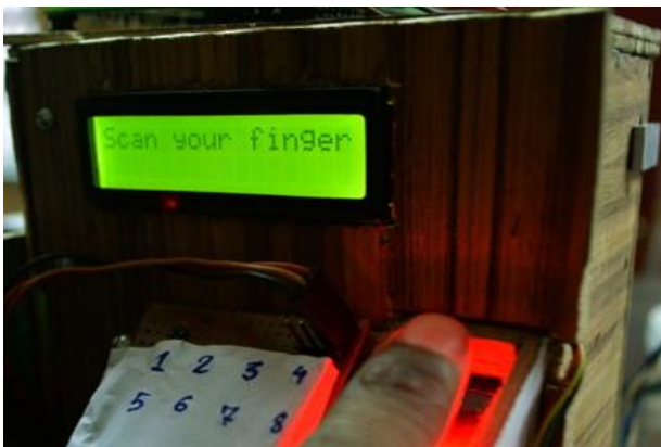
Fig. 6. Status of the security system when the system scans the finger of the person for finger-print verification.
