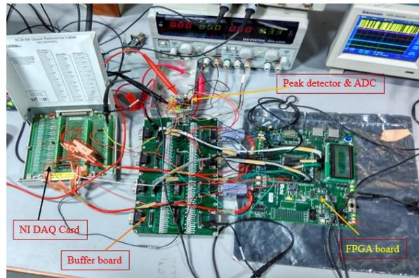
Fig. 16: Hardware Connections of Processing Electronics
