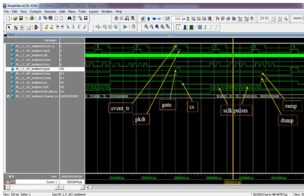
Fig. 4. Simulation results of Method-1 FPGA code
