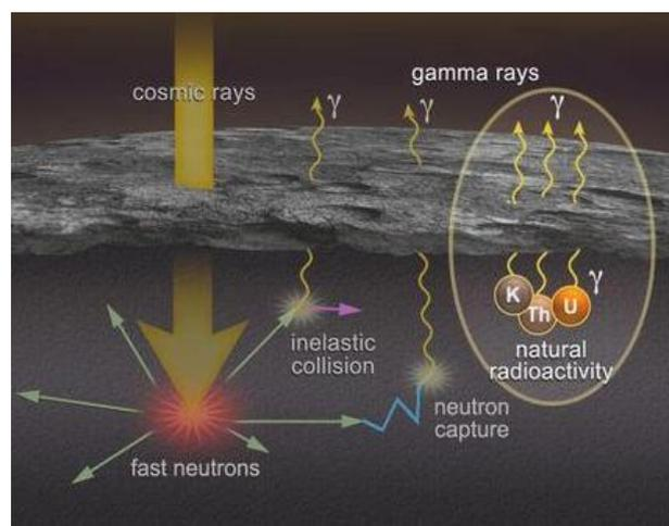
Fig. 1: Generation of the  $\gamma$  - rays
