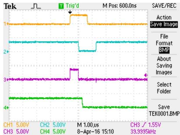
Fig. 13: CRO reading-1 of Method-2 (event trigger pulse (orange), PKDT control signal of peak detector (blue), gate control signal of peak detector (pink), CS conversion start signal of ADC (green))
