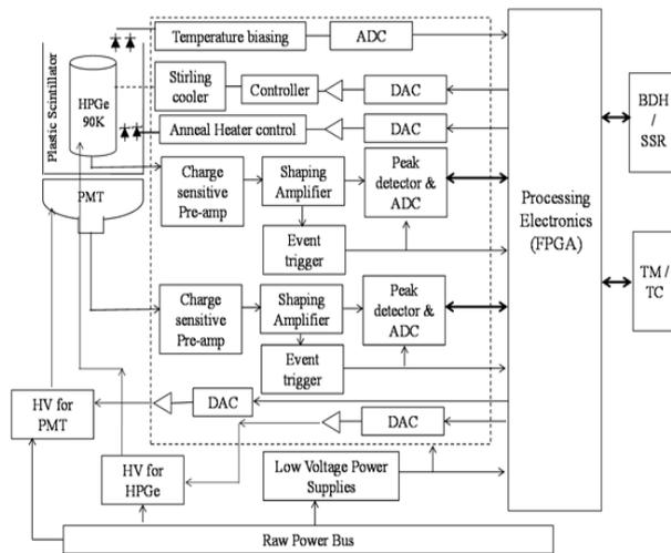
Fig2. Block diagram of GRS
