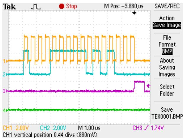
Fig. 14: CRO reading-2 of Method-2 (SCLK pulses (yellow), output of ADC (blue), CS signal of ADC (pink), synchronization clock between FPGA & LabVIEW (green))
