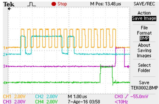
Fig.5. control signals of CRO readings of Method-1(SCLK pulses (yellow), output of ADC (blue), conversion start signal of ADC (pink), synchronization clock between FPGA & LabVIEW (green))
