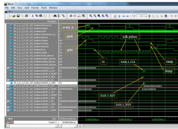
Fig. 9: Simulation result-1 of Method-2 FPGA code
