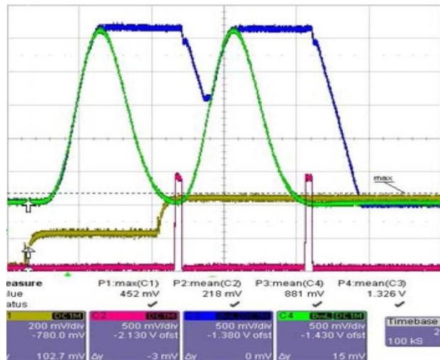
Fig.3. CRO reading of input & output signals at peak detector [1] (output of the shaper (green), output of the peak detector (blue), peak discharger pulse (red), input test signal (yellow))
