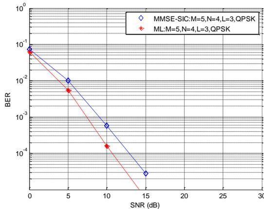
Figure 5.1 M=5, N=4, L=3, QPSK modulation with ML & MMSE-SIC equalizer
