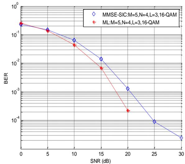
Figure 5.3 M=5, N=4, L=3, 16-QAM modulation with ML & MMSE-SIC equalizer
