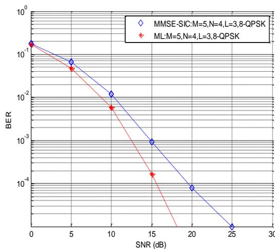
Figure 5.2 M=5, N=4, L=3, 8-QPSK modulation with ML & MMSE-SIC equalizer
