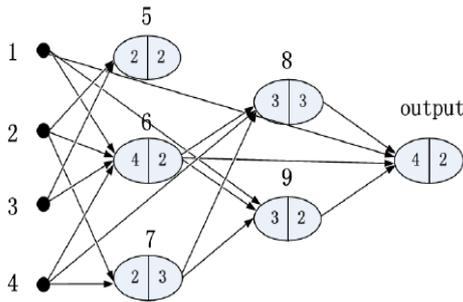
Fig 6. The structure of the EA-GMDH network
