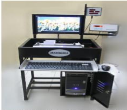
Figure 1. PC based Automatic Milk Collection Unit
