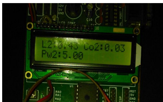
Figure 7: Intensity of light and CO2 emission (in ppm) when 5W LED bulb is used.
