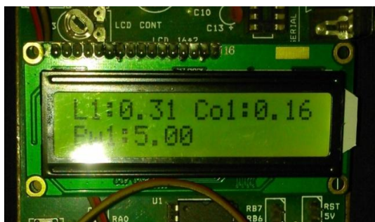
Figure 6: Intensity of light and CO2 emission (in ppm) when 5W Incandescent bulb is used
