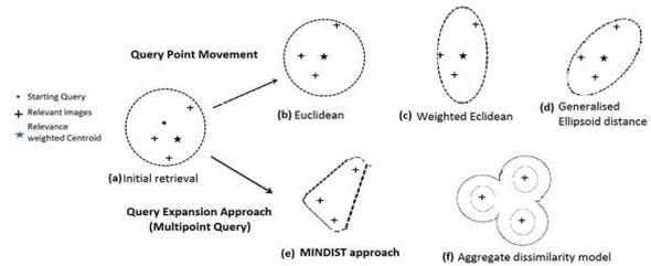
Fig. 3: Query vector movement and Query expansion shown along with the iso-curves for each of the distance measures
