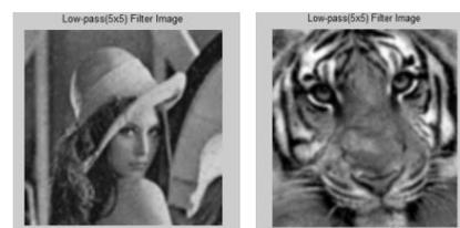
Fig 4.8 Low pass (5\*5) filter image
