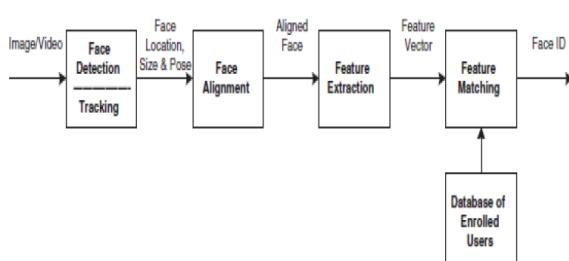
Figure 1: Face Recognition processing flow
