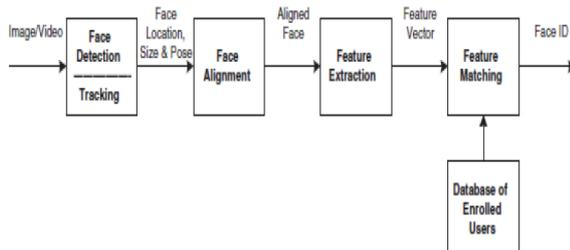
Figure 1: Face Recognition processing flow
