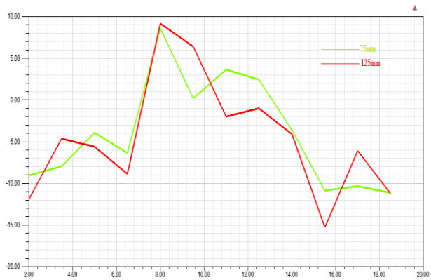
Fig24: Gain varied with tapered slots length of QETSVA
