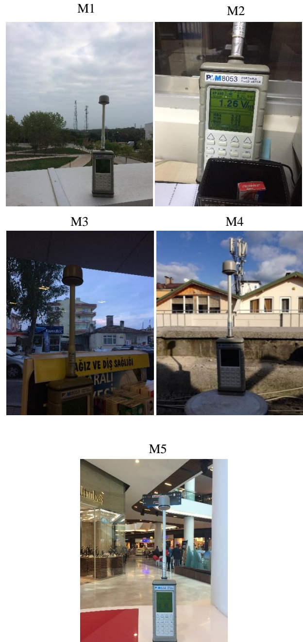
Fig. 2. Pictures of E measurements at different locations using PMM-8053 EM field meter
