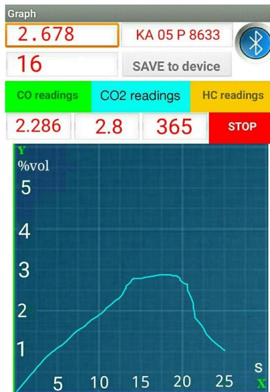
Fig. 16 CO<sub>2</sub> emission of the vehicle with registration number “KA 05 P 8633” tested using Electronic Nose
