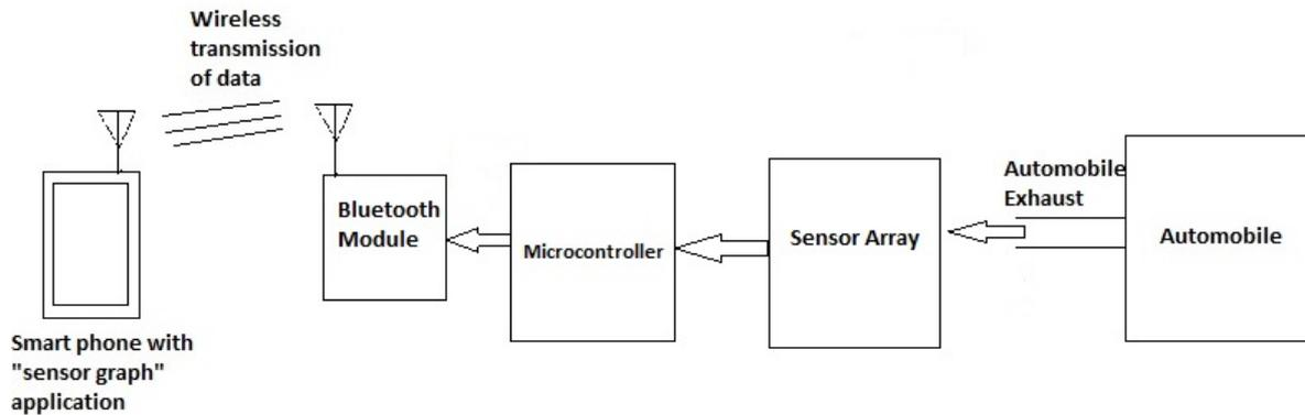
Fig. 4 General block diagram of electronic nose
