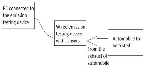
Fig 1 Block diagram of existing emission testing system
