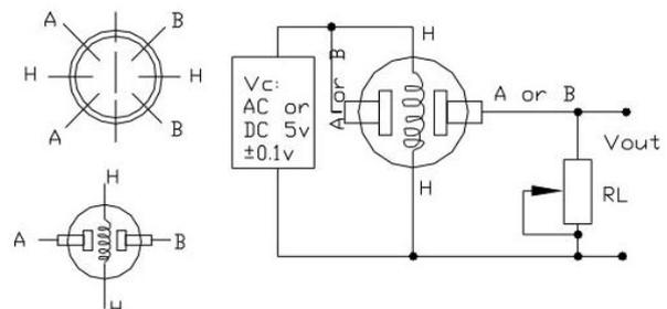
Fig. 7 General circuit connections of MQ sensor
