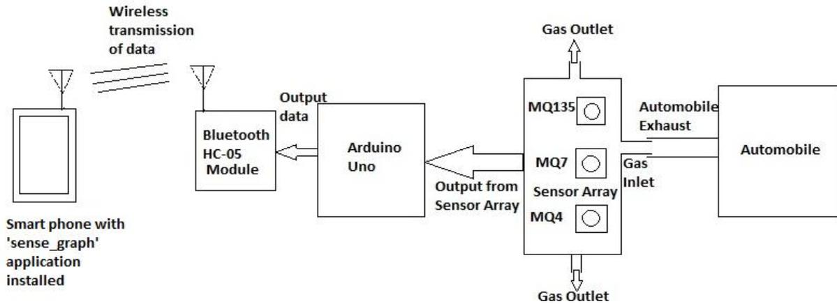
Fig. 12 Detailed block diagram of electronic nose
