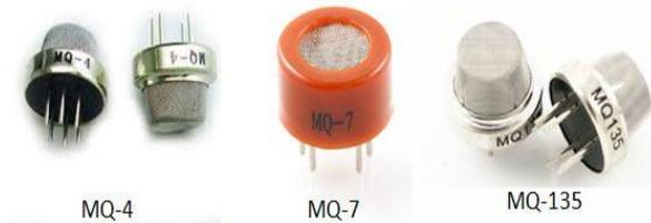
Fig. 5 MQ-4, MQ-7 and MQ-135
