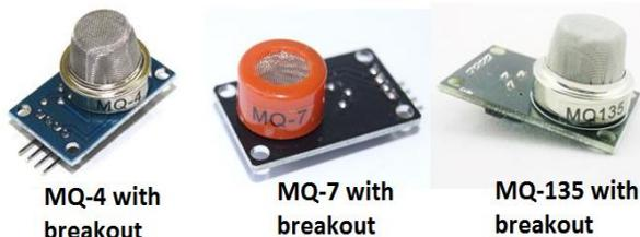
Fig. 6 MQ-4, MQ-7 and MQ-135 with their respective breakout circuits
