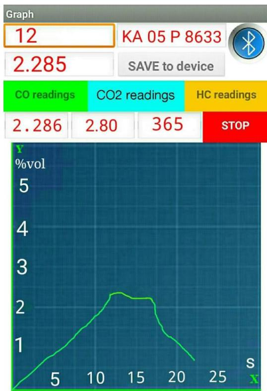
Fig. 15 CO emission of the vehicle with registration number “KA 05 P 8633” tested using Electronic Nose
