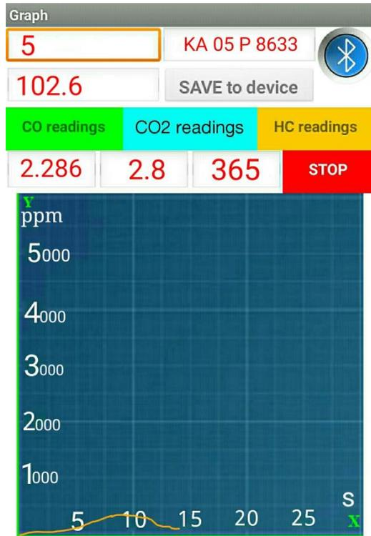
Fig. 17 HC emissions of the vehicle with registration number “KA 05 P 8633” tested using Electronic Nose.
