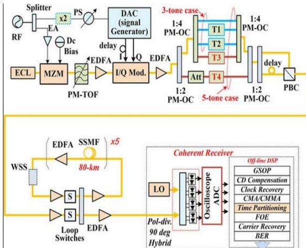
Fig 2: 110 GBaud QPSK signal generation, transmission and coherent detection system.
