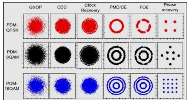
Fig4: The constellation of different signals after 1000-km transmission with DSP
