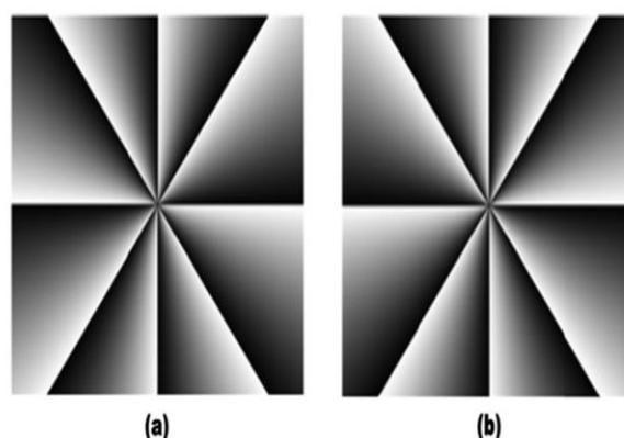
Fig7: SLM hologram pattern with charge of (a) +8 and (b) -8
