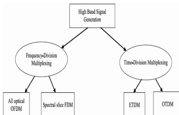
Fig.1 : High baud rate signal generation by FDM and TDM methods reported in previous work
