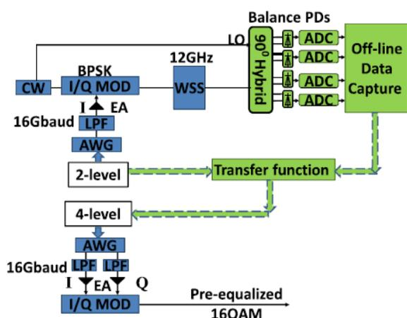
Fig6: The principle of pre-equalization.
