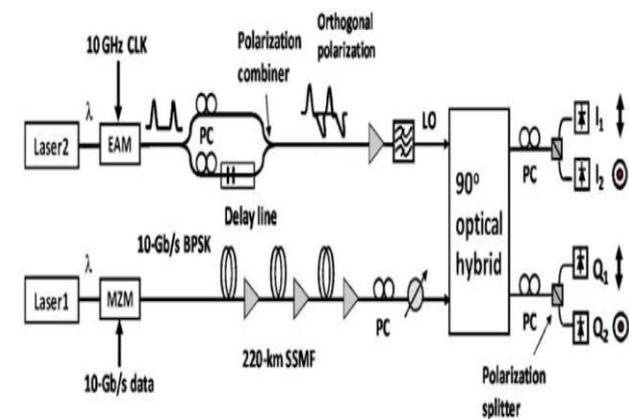
Fig.9. Experimental setup for COTDS
