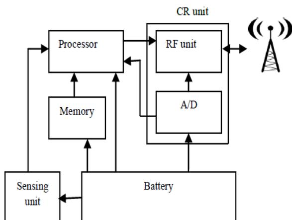
Fig. 5 Hardware Structure of a Cognitive Radio Sensor node
