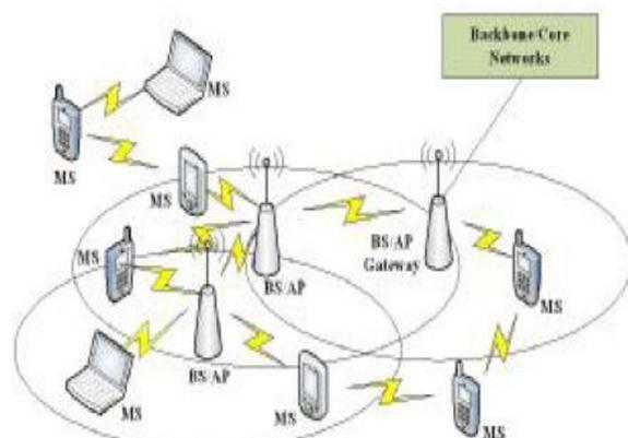
Fig.4. Mesh Architecture Network
