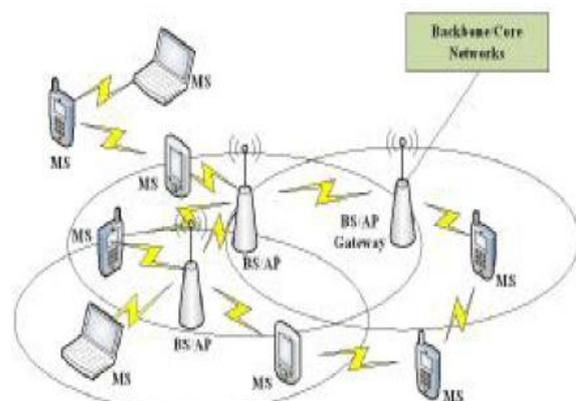
Fig.4. Mesh Architecture Network
