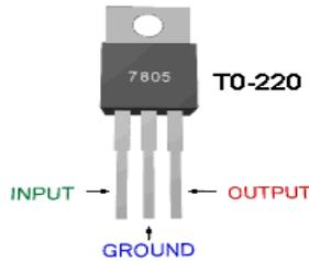
Fig; Pin diagram of IC7805
