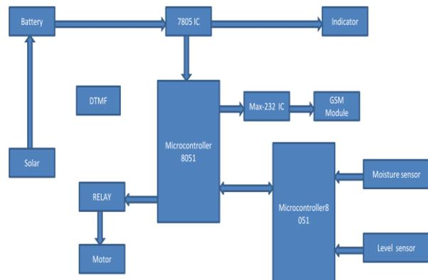
Fig: Block Diagram of Model
