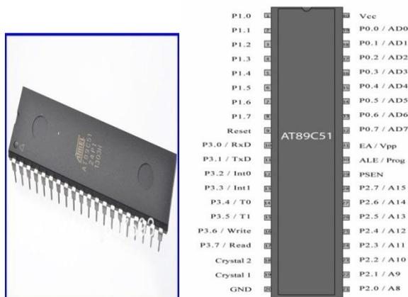
Fig; AT89C51 IC Fig; Pin Description
