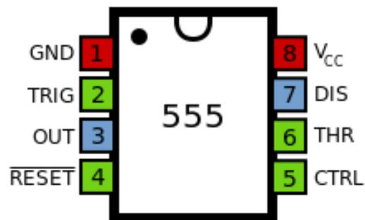
Fig; IC555 Pin diagram
