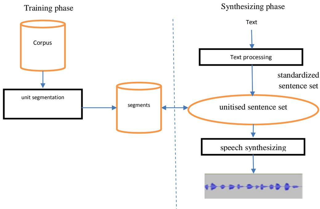
Figure 6: Text-to-speech procedure by connecting to unitise.
