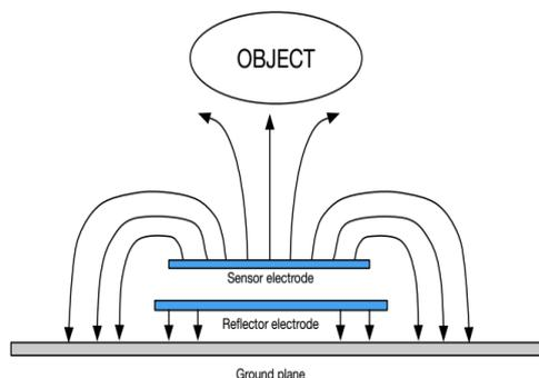
Fig. 1. The structure of a capaciflector depicting the three electrodes and direction of electric flux.
