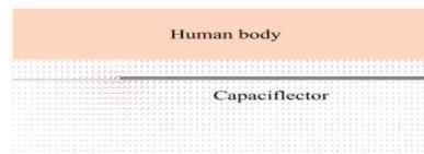
Fig. 4. A simulation of the capaciflector showing the effect of an object on the electrical flux surrounding the device.
