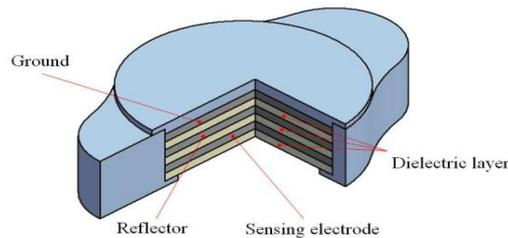
Fig. 2. An exploded view of the capaciflector showing the electrode and dielectric layers, together with the 3D printed housing (not to scale)
