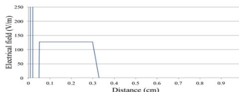
Fig. 5. A plot of electric field strength along the central axis outwards from the capaciflector. (Note that the plot has been truncated to remove the peak between the reflector and ground electrodes.)
