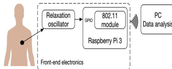
Fig. 6. A system block diagram of the test setup showing the capaciflector mounted on the chest, the front-end electronics and the remote data analysis capability provided by a WiFi connection.
