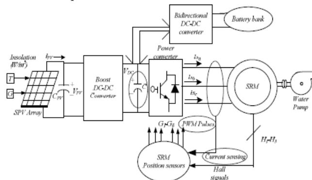
Fig.1. Conventional SPV+ battery fed SRM driven water pumping system
