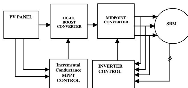
Fig.2. Proposed SPV fed SRM driven water pumping system utilizing Boost converter
