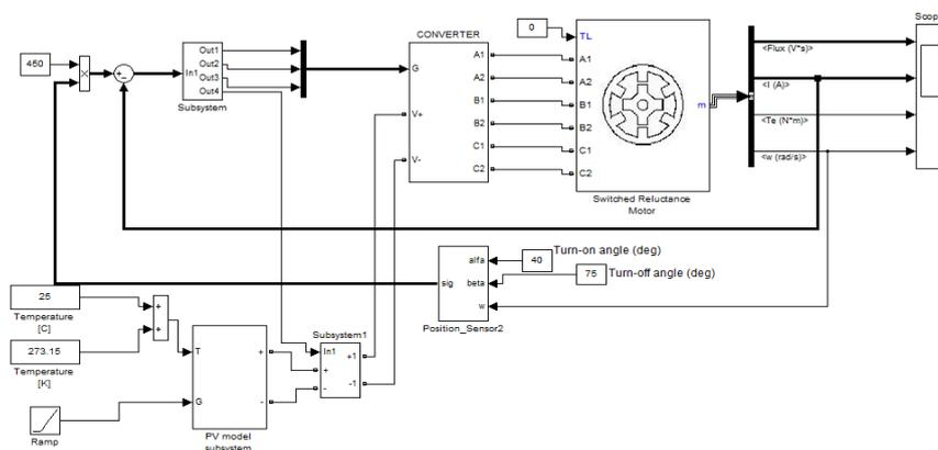
Fig.4 Developed simulink model of SRM
