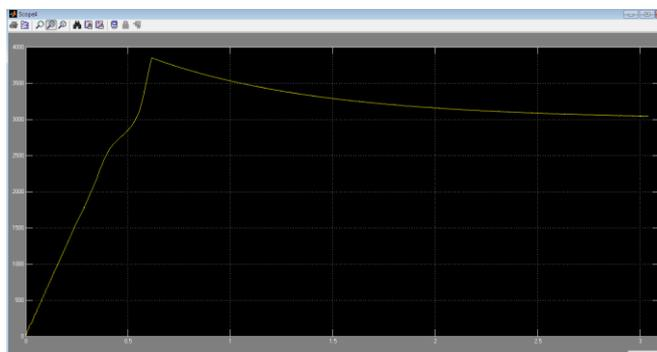
Speed of the motor in rotation per minute.
