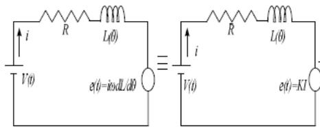
Fig. 3 Equivalent circuit of SRM
