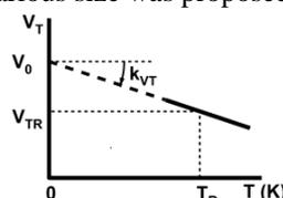
Figure 2: temperature dependence of threshold voltage  $V_t$
