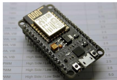
Fig. 5. Node MCU hardware
