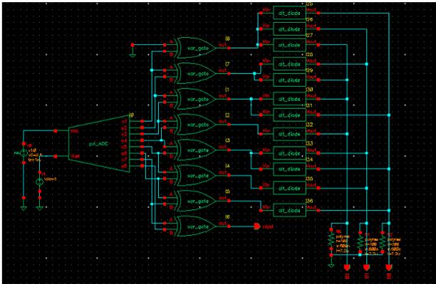
Fig. 2 schematics of flash ADC
