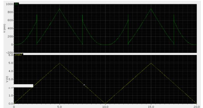
Fig. 6 output waveform of folding technique in flash ADC
