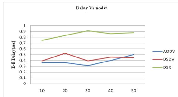
Fig. 2 Average End To End Delay Vs. Number of Nodes
