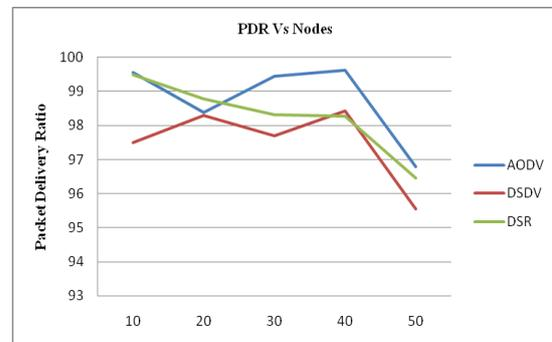
Fig. 3 Packet Delivery Ratio vs. Number of Nodes
