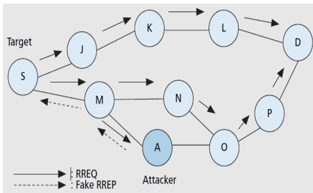
Figure1. Example of blackhole attack on AODV
