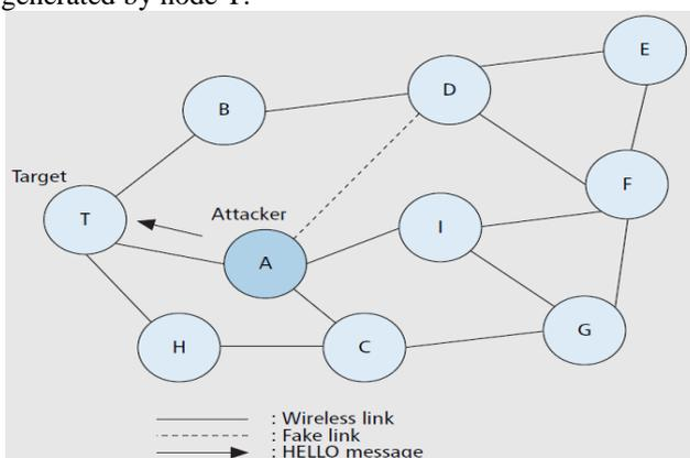
Figure 2. Example of link spoofing attack on OLSR
