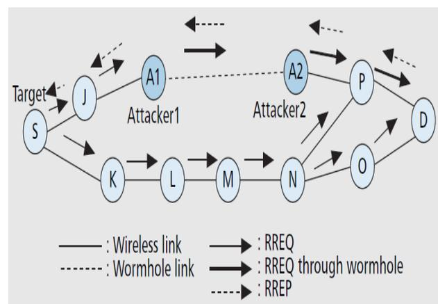
Figure 3. Example of wormhole attack on reactive routing
