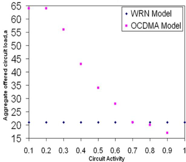
Fig. 7. Aggregate offered circuit load Vs Circuit activity with  $K = 64$  subscribers,  $\Gamma = 32$  channels  $p_{outage}^{max} = 10^{-6}$  and  $p_{blocking}^{max} = 10^{-2}$ .
