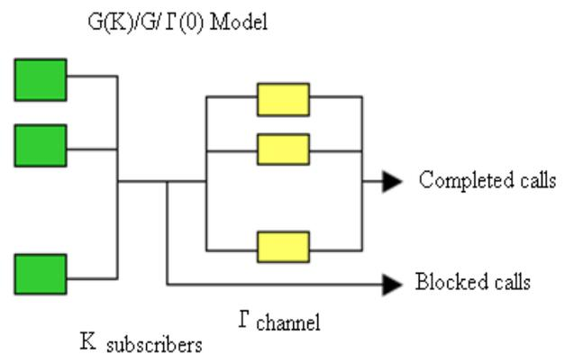
Fig.2. WRN model with K subscriber;  $\Gamma$  available wavelength
