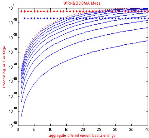
Fig. 6. Plot for  $P_{outage}$  or  $P_{block}$  Vs aggregate offered circuit load with  $K = 64$  subscribers,  $\Gamma = 32$  channels  $p_{outage}^{max} = 10^{-6}$  and  $p_{blocking}^{max} = 10^{-2}$ .
