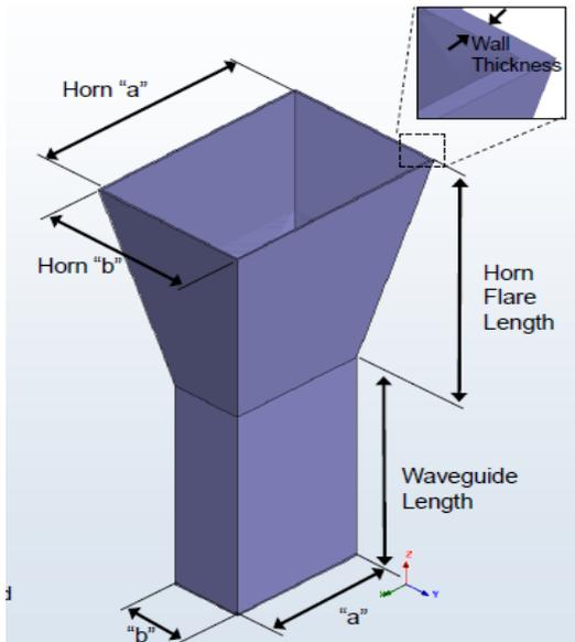
Fig.1 Structure of Proposed Horn Antenna
