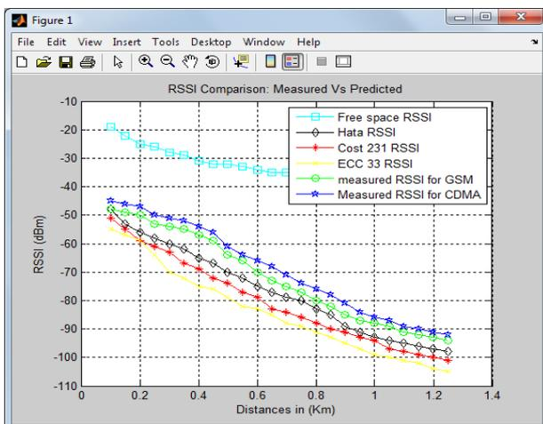
Figure 11: RSS Comparison – Measured Vs Predicted (Traditional Models)
