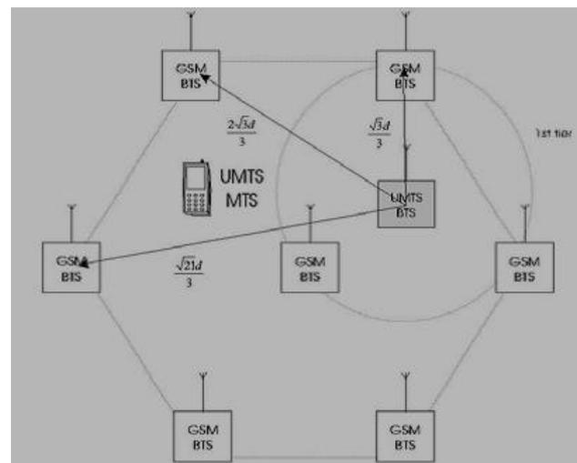
Figure 7: Multiple GSM900 Base Stations causes IM interference to UMTS800 Base Stations or Mobile Stations (uncoordinated Operations)
