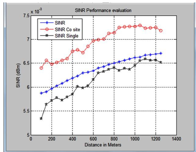
Figure 12: Simulation of SINR performance evaluation
