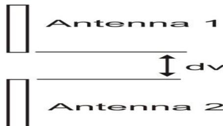
Figure 2: Antenna configuration for vertical separation (co-location)
