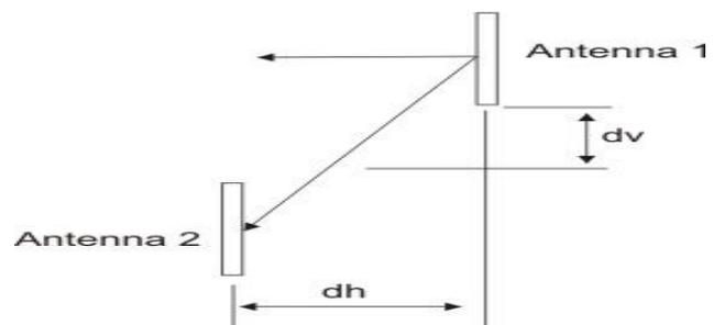
Figure 4 :Antenna configuration of slant separation
