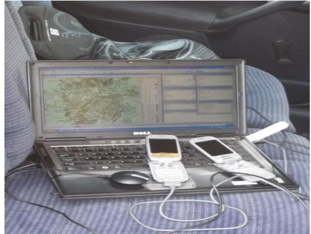
Figure 6: TEMS Measurement Tool used for Field gathering of RSS Data
