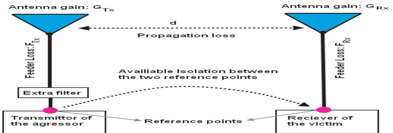
Figure 9: Design for Antenna Isolation Measurements
